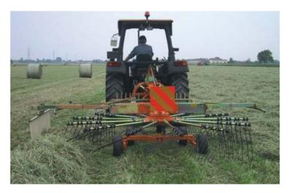
To assist in all conditions there is a variable tine bar cam, easily adjusted to ensure a clean sweep of all crops.
